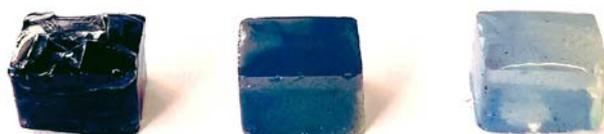
**Figure 4:** Pictures of hydrogels containing different amount of PEDOT-N polymers.
