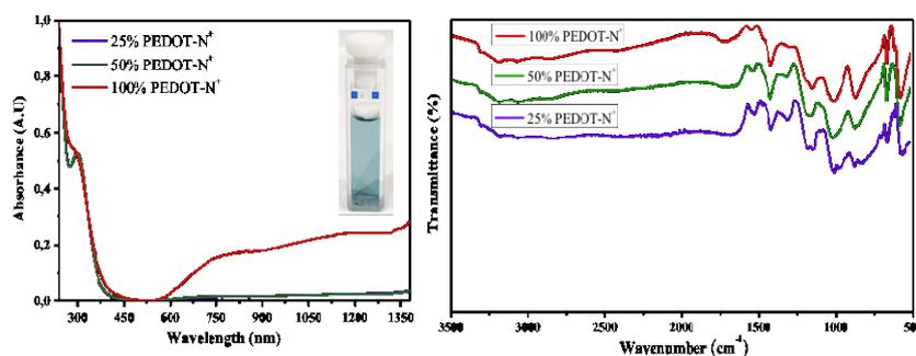
**Figure 1:** Left side, UV-VIS spectra of aqueous solution of PEDOT-N copolymers and right side, FTIR spectra of PEDOT-N copolymers
