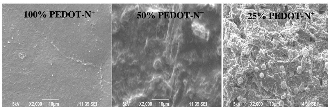
**Figure 3:** SEM images of films obtained from PEDOT-N and PEDOT-N-PEDOT copolymers having 50% EDOT-N units and 25 % EDOT-N units respectively
